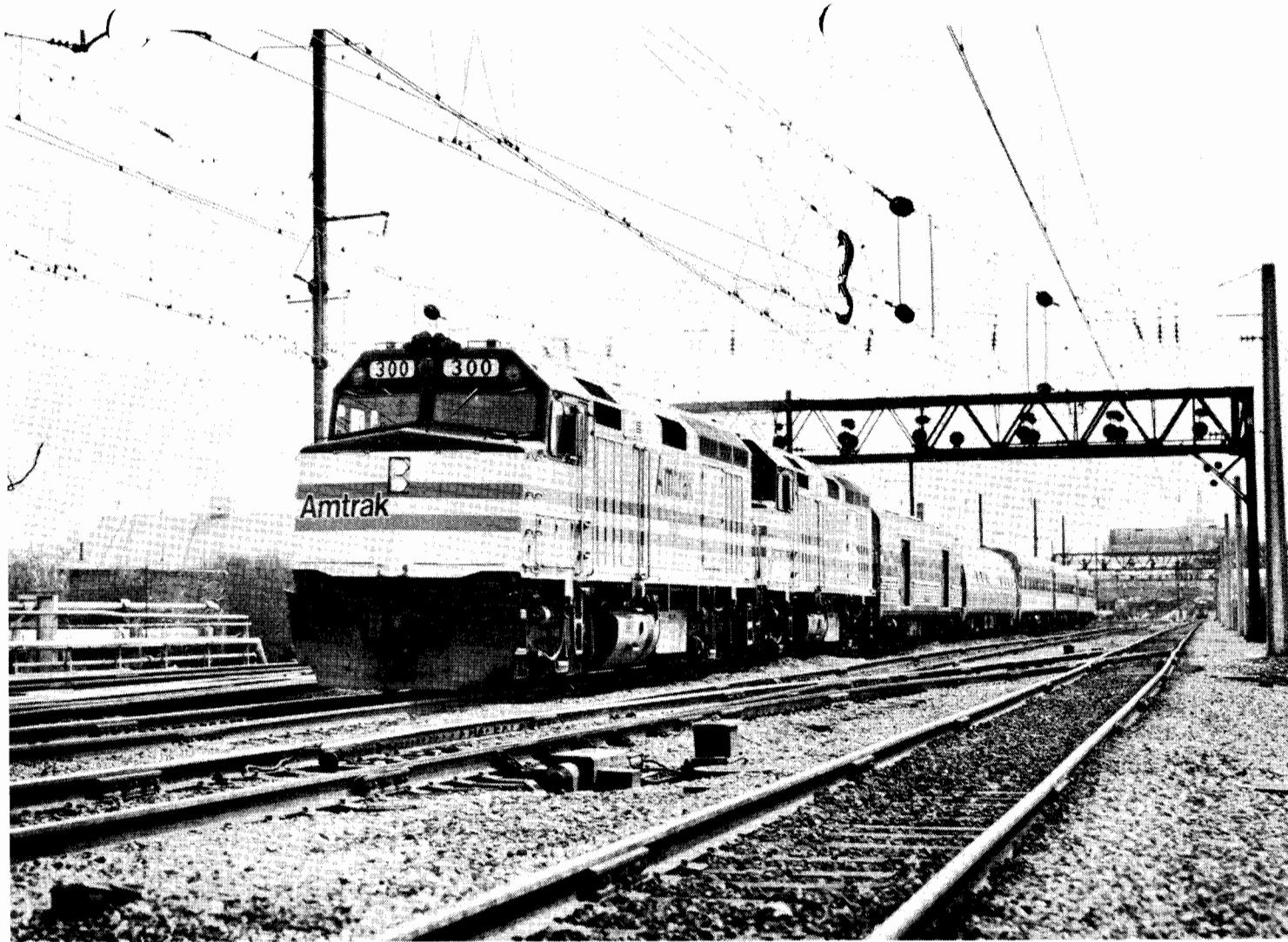
The Washington section of a head end power-equipped Broadway Limited---with diesel locomotives under the catenary---leaves Washington's Union Station for Chicago. The Broadway was the second Amtrak train---the Lake Shore Limited was the first---to be completely equipped with head end powered cars. (Amtrak Photo)
